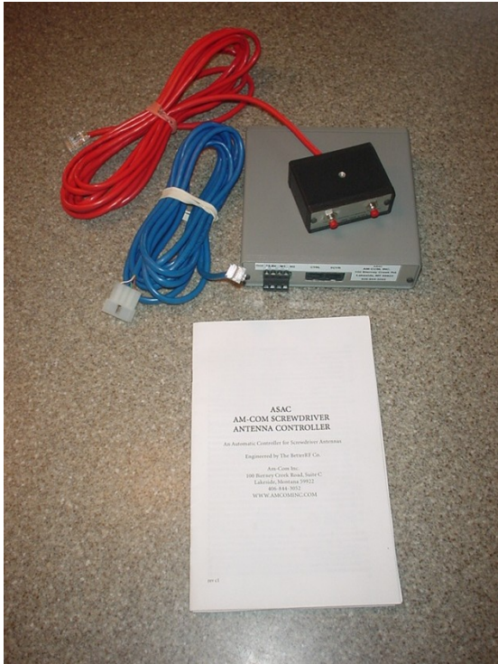
AM-COM ASAC-100 controller – used for mobile operation of the HS-1500 antenna
